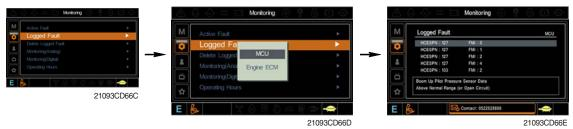
$\cdot\,$  The logged faults of the MCU or engine ECM can be checked by this menu.
